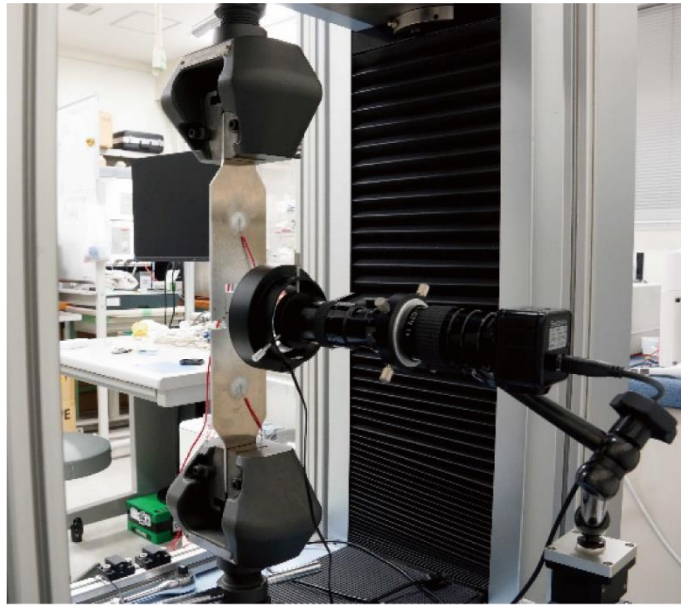
Fig. 2.2 Tensile shear testing with a bonded plate specimen. Deformation in the adhesive layer is measured by microscope.
