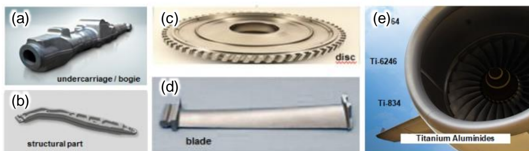
Fig. 1.2 Examples of titanium alloy applications for aircraft 11) : (a) undercarriage, (b) structural part, (c) turbine disc, (d) turbine blade and (e) turbine engine.
