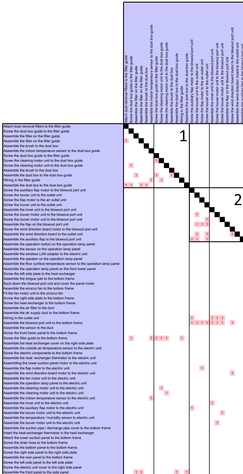
Fig. 4.16 Assembly process DSM partitioning result of the air conditioner [left half part].
