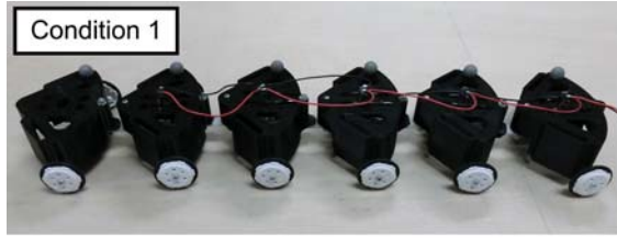
(a) Ground contact condition 1 with dynamical fore-hind symmetry: all the passive wheels touch the ground
