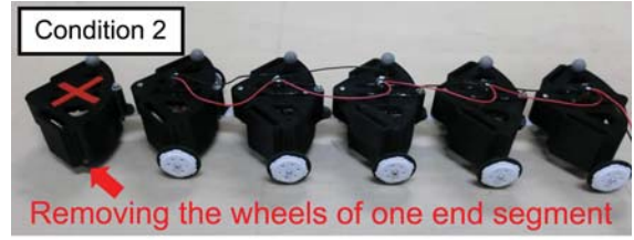
(b) Ground contact condition 2 with dynamical fore-hind asymmetry: the wheels of one end segment are removed
