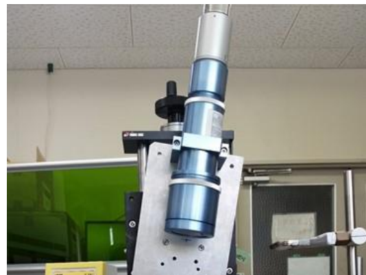
(b) Laser processing head
