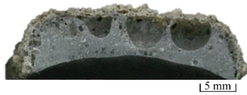
Fig. 2.12 Example of cross-section of slag.
