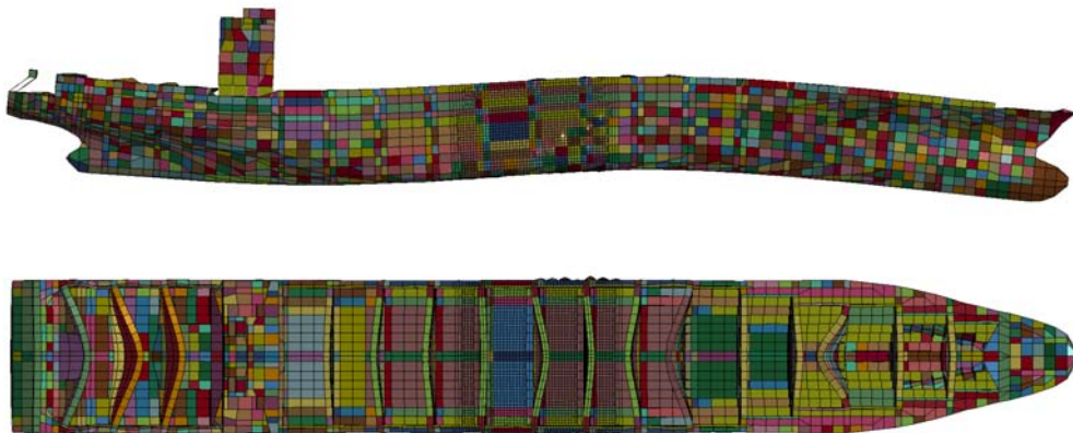
Figure 4.20 3-node vibration mode shape of prototype full scale ship FEA model (1.28Hz)
