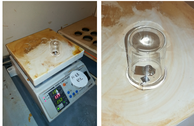
Figure 2.6: The wafer is under HMDS treatment. The copper cup is made of a copper plate and copper pipe. This treatment should be done in a draft chamber because heated HMDS generates ammonium gas.
