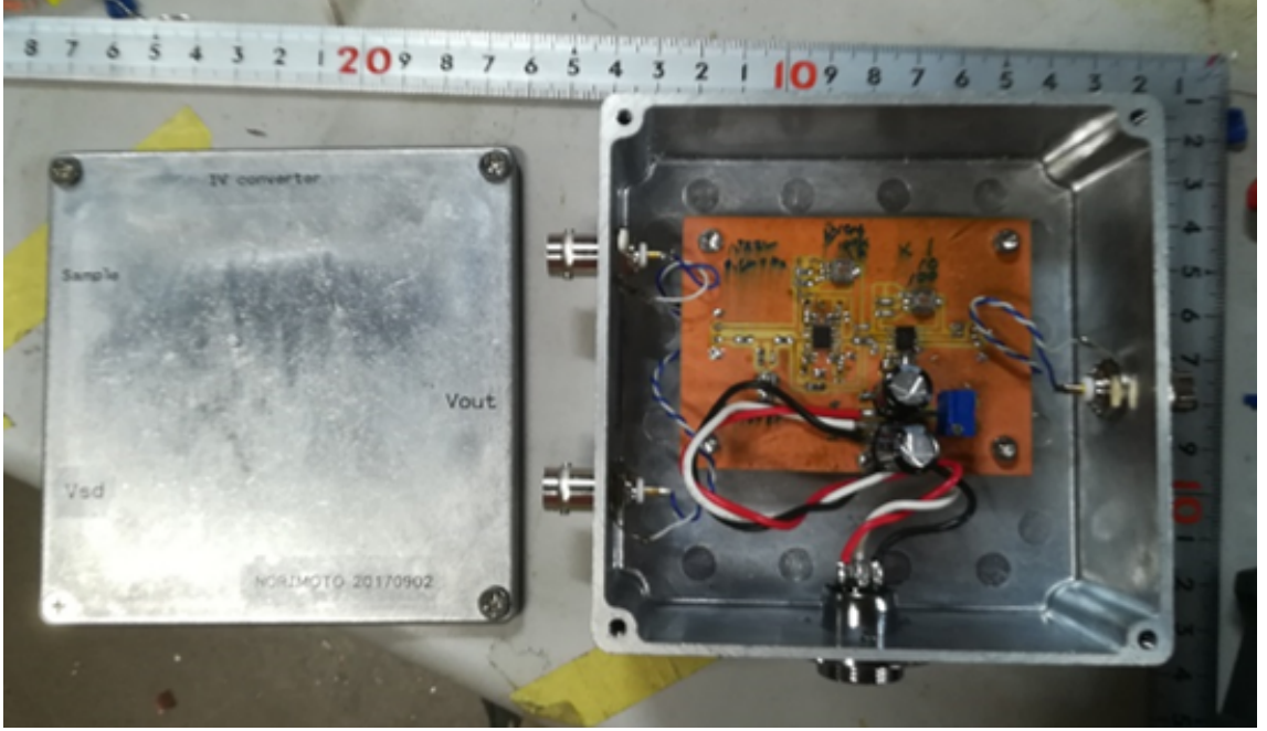
Figure 5.8: A photo of homemade current-voltage converter.
