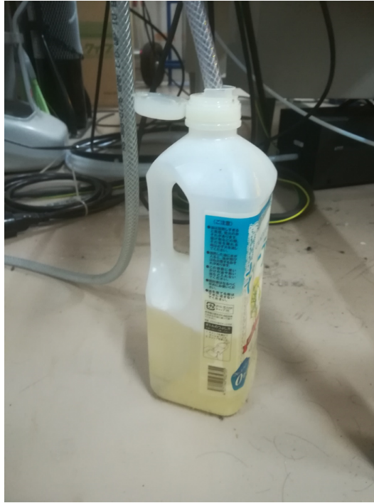
Figure 2.9: How to keep furnace 1 atm. After flushing, the output port is put into oil to keep furnace at 1 atm. Then all ports are closed.
