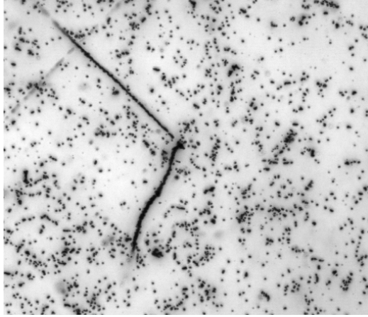
Figure 5.2: Photograph of the end point of track #8. Track #8 came to rest from the bottom. A charged particle was emitted to the upper-left direction.
