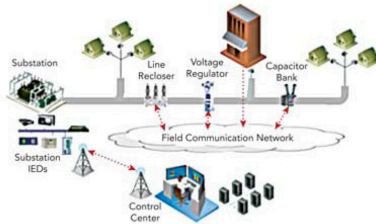
Figure 1.2: An illustration of a Distribution Automation System [10].
