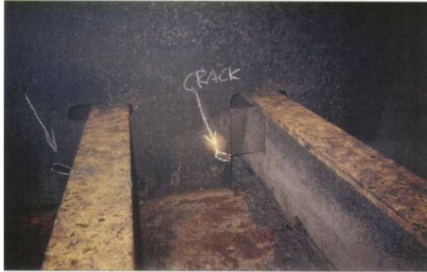
(a) fatigue cracks in way of the longitudinal cutouts.
