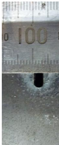
Fig. 3.6 Steel plate specimen cutting groove. (a) 100%H 2 -0%CO 2 . (b) 80%H 2 -20%CO 2 .
