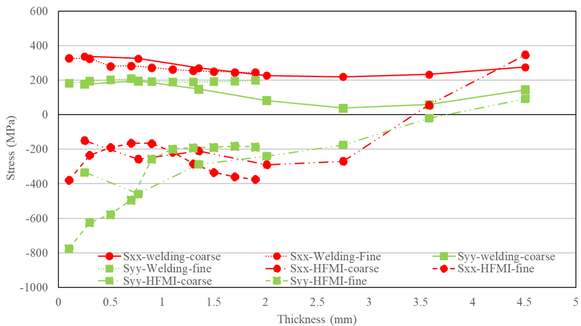
Fig. D-1 Residual stress comparison between coarse and fine model.
