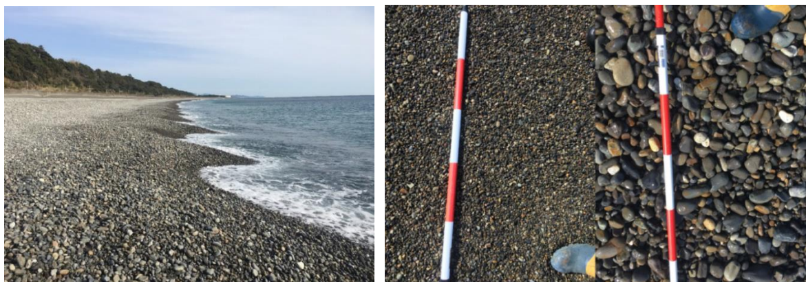
Figure 2.17 Left: Cusp formation in the winter season Right: a) the particle between the cusps, b): the particle on the cusp
