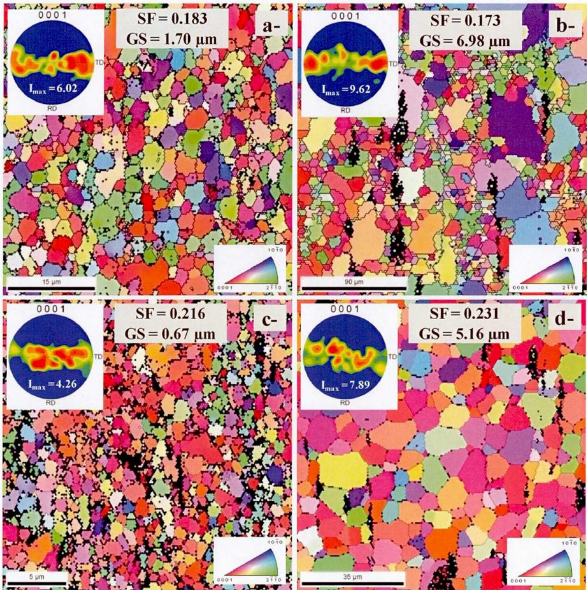
Fig. 4.10 The EBSD analysis results of (a) AMX602 alloy SWAP powder, (b) AMX602 alloy cast, (c) ZAXE1711 alloy SWAP powder, and (d) ZAXE1711 alloy cast specimens extruded at 673 K showing both the crystal orientation mapping and the basal plane orientation texture.
