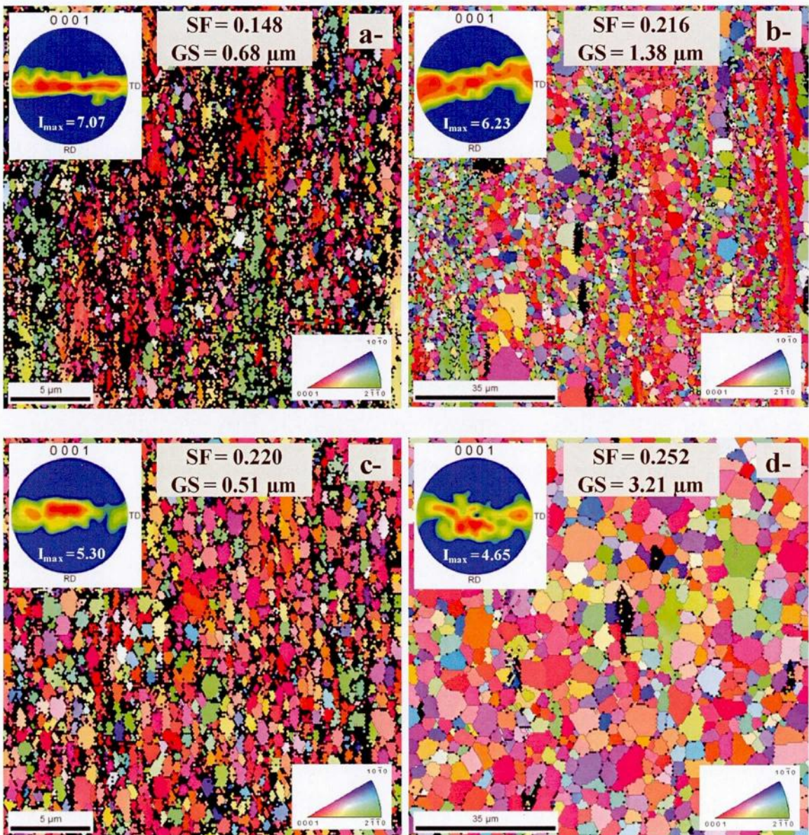
Fig. 4.12 The EBSD analysis results of (a) AMX602 alloy SWAP powder, (b) AMX602 alloy cast, (c) ZAXE1711 alloy SWAP powder, and (d) ZAXE1711 alloy cast specimens extruded at 573 K showing both the crystal orientation mapping and the basal plane orientation texture.
