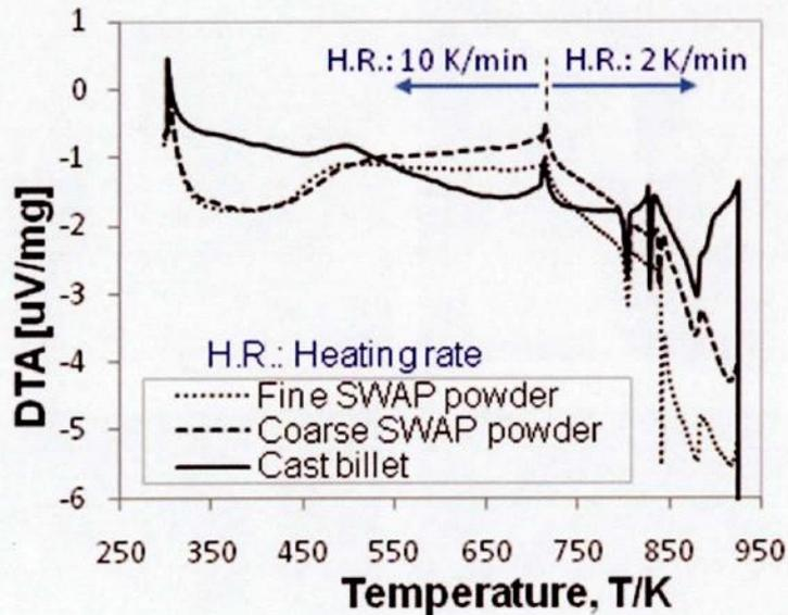
Fig. 3.10 DTA pattern of AMX602 alloy raw materials.
