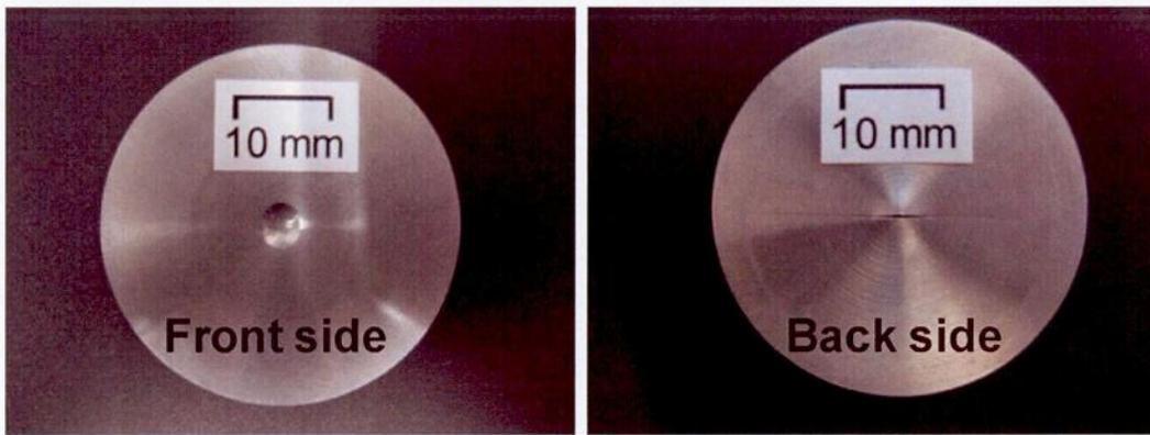
Fig. 7.11 The deformation of ballistic impact test specimen.
