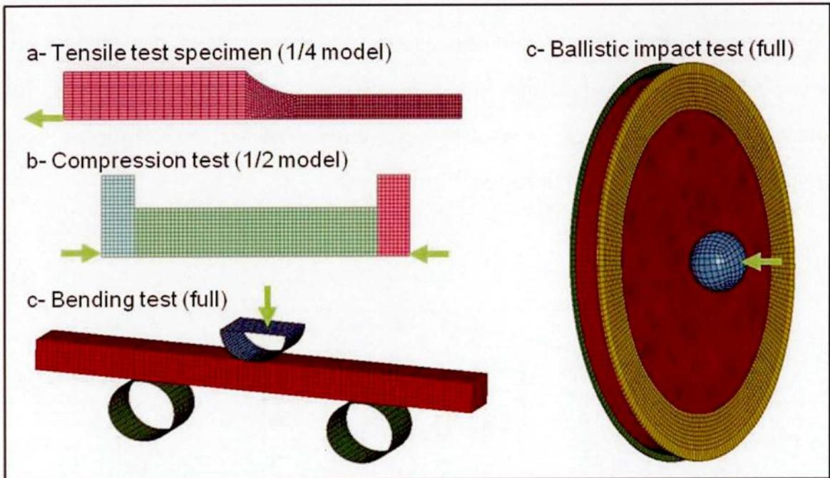
Fig. 2.9 Models for FEM analyses showing the mesh distribution.
