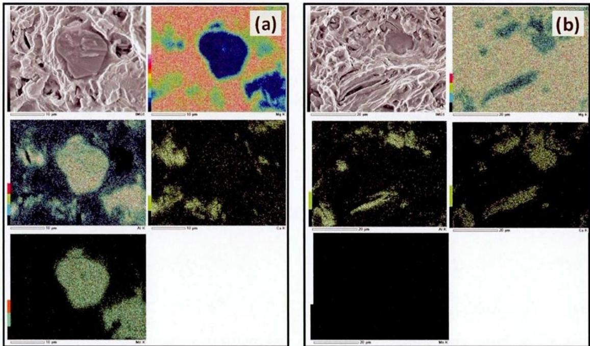
Fig. 6.5 EDS analysis of the fracture surface of tensile test specimen of cast billet extruded at 673 K showing both Al-Mn (a) and Al-Ca (b) compound particles.
