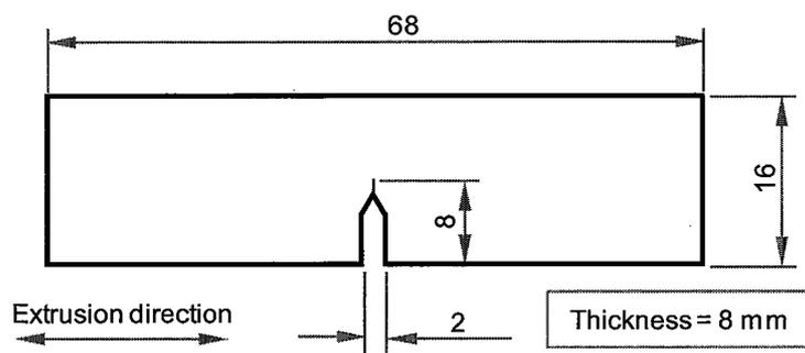
Fig. 6.1 fracture toughness 3-point bending specimen.
