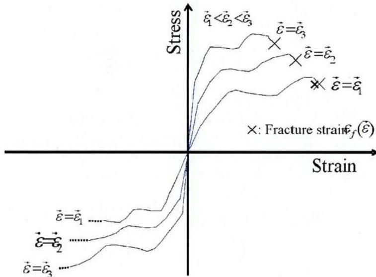
Fig. 7.4 Independent stress-strain curves for tension and compression at different strain rates [14].
