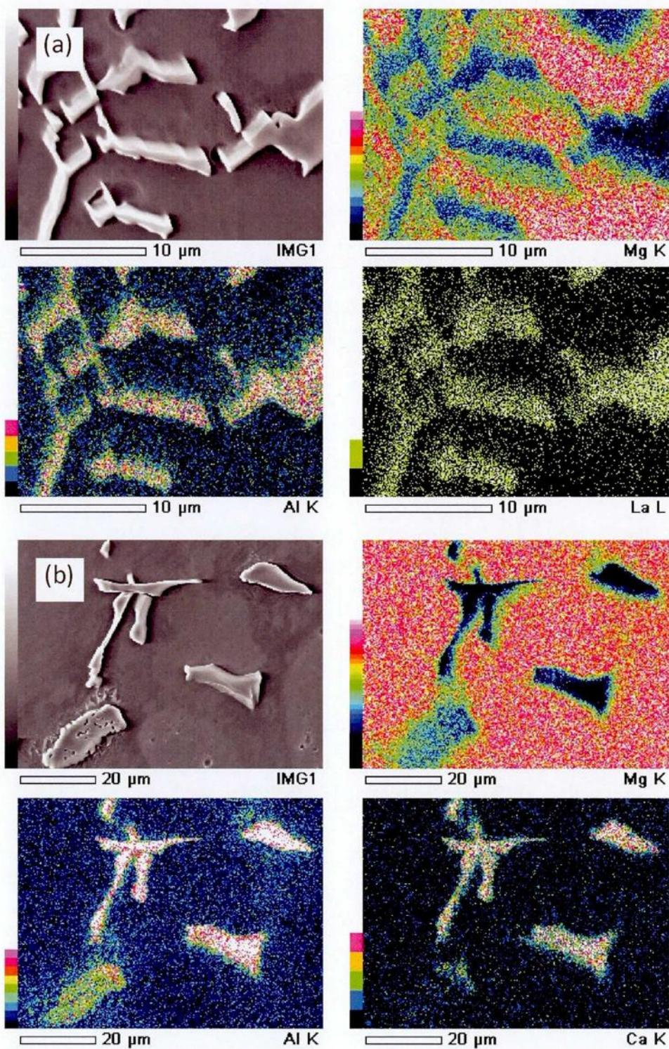
Fig. 3.7 EDS analysis of cast ZAXE1711 alloy showing both  $Al_{11}La_3$  (a) and  $Al_2Ca$  (b) intermetallic compounds.
