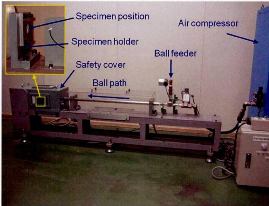
Fig. 2.7 Ballistic impact test specimen and setup.
