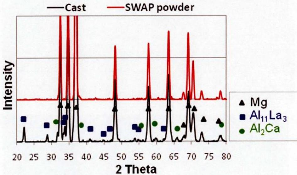
Fig. 3.6 XRD patterns of ZAXE1711 alloy SWAP powder and cast.
