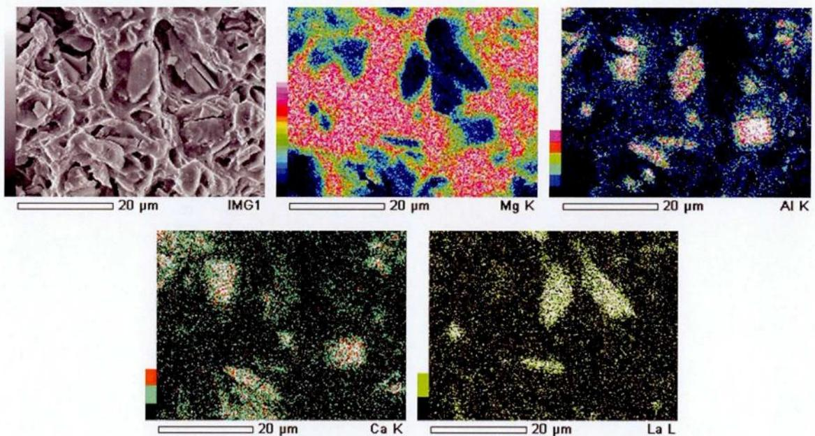
Fig. 5.10 EDS of fracture surface of tensile test specimen of ZAXE1711 cast alloy extruded at 573 K.
