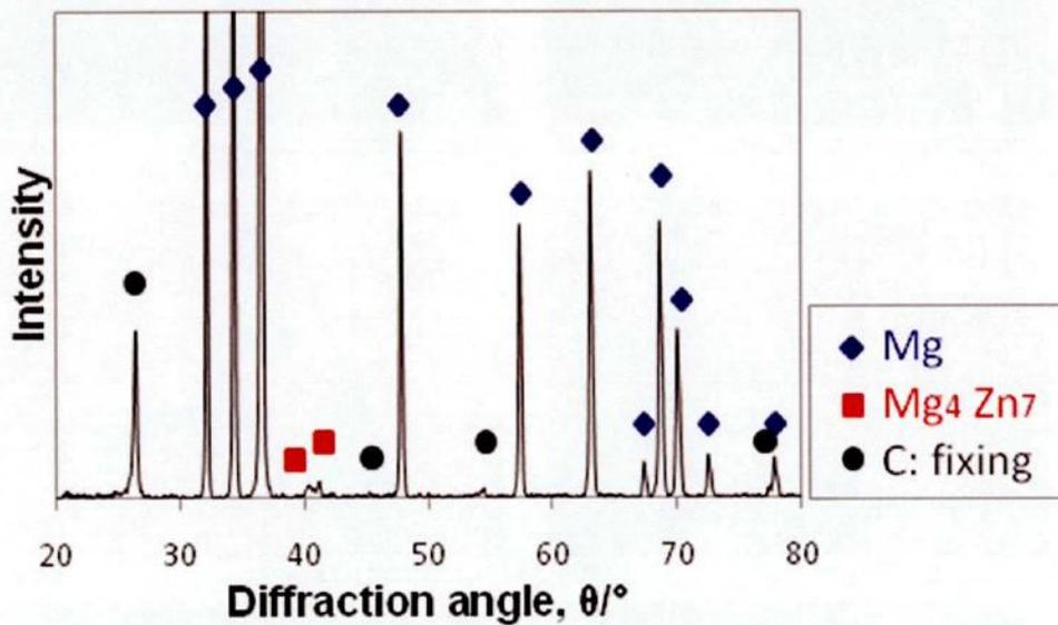
Fig. 3.8 XRD patterns of atomized ZK61 alloy powder.
