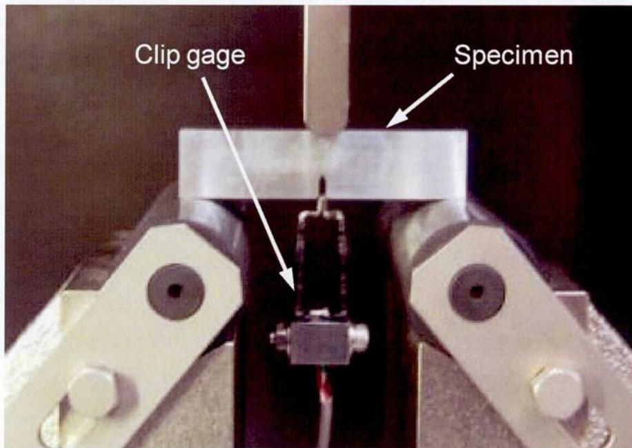
Fig. 2.6 Fracture toughness test specimen and setup.
