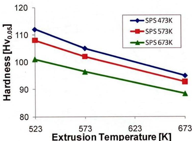
Fig. 5.12 Hardness of extruded ZK61 alloy atomized powder.
