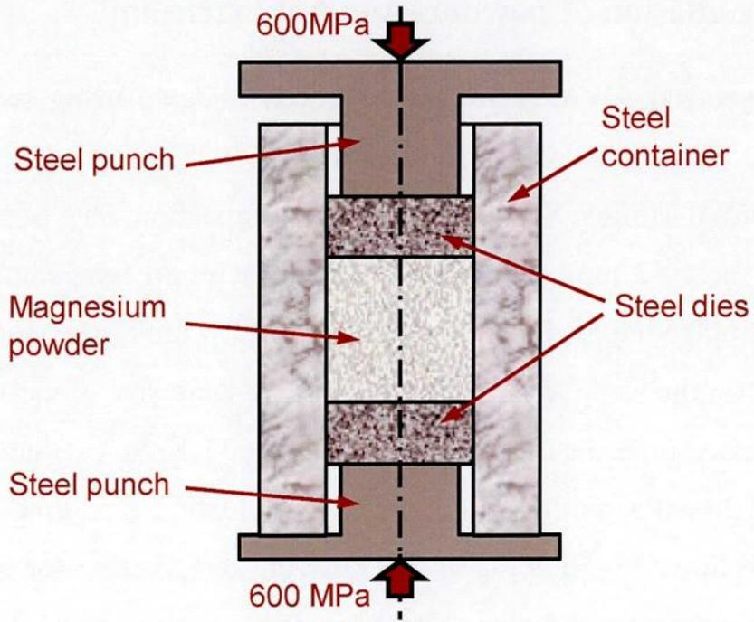
Fig. 2.2 Schematic illustration of the cold compaction process.
