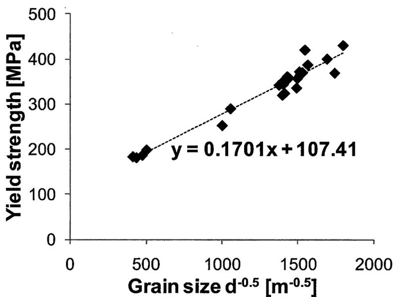
Fig. 5.8 Hall Petch relationship of extruded ZAXE alloys.
