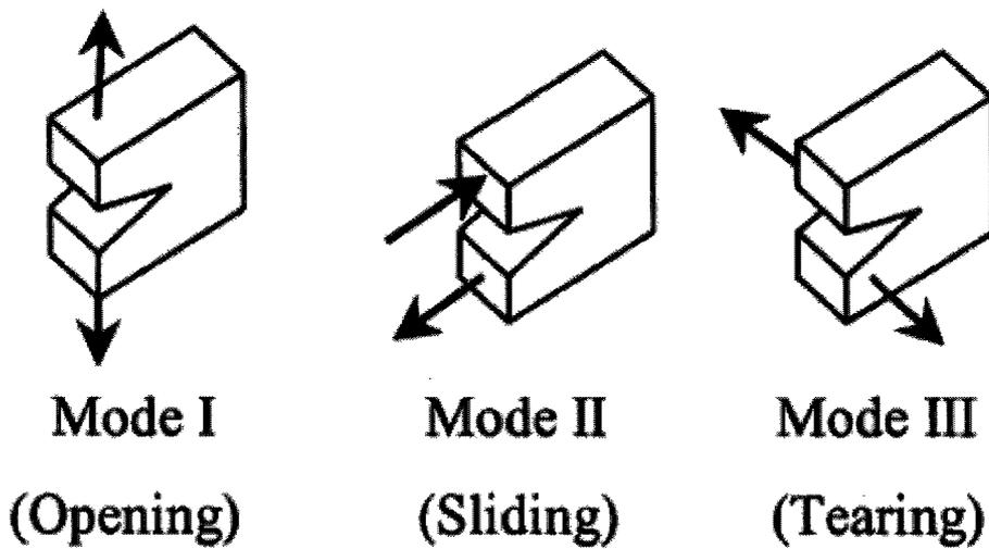
Fig. 1.2 The three loading modes of the cracked components [67].
