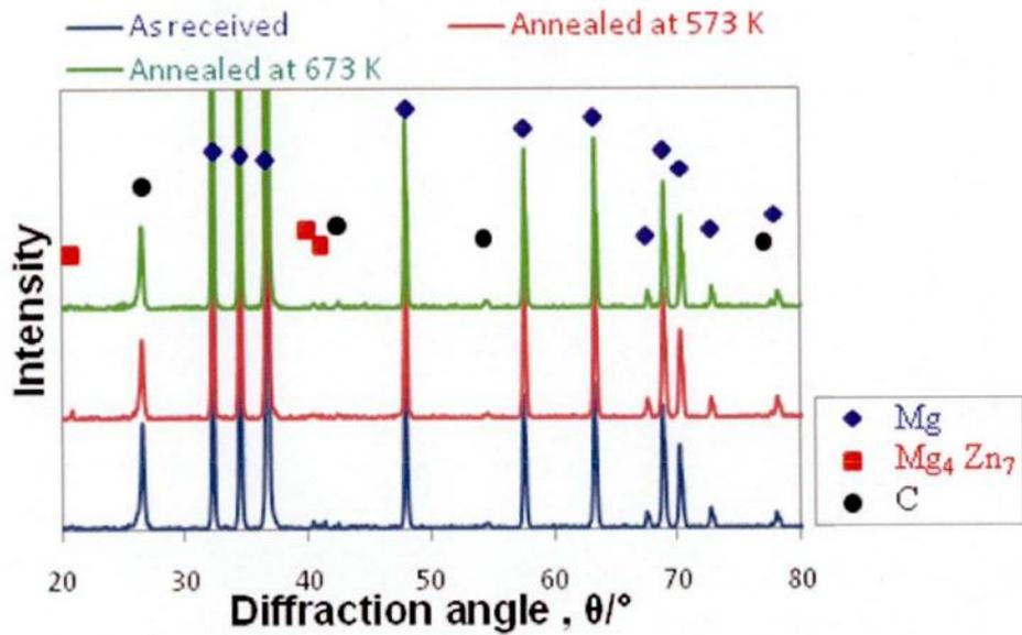
Fig. 3.17 XRD of ZK61 alloy powder annealed at various temperatures.
