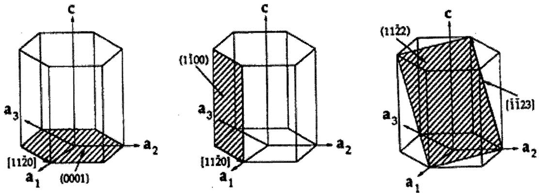
Fig. 1.1 The hexagonal close packed (hcp) crystal structure [1].
