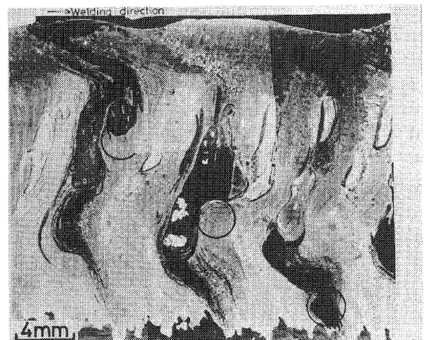
Photo. 11 Solidification pattern of segregation region in longitudinal section of SUS304N welds. (Used aluminum brazing filler metal for insert metal)
