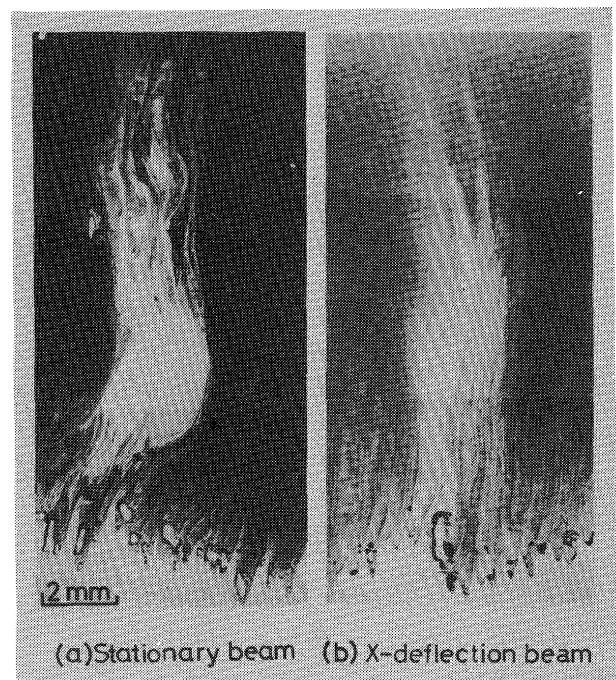
Photo. 8 Solidification pattern of longitudinal section of SUS304 welds. (Used covered electrode core wire for insert metal)
