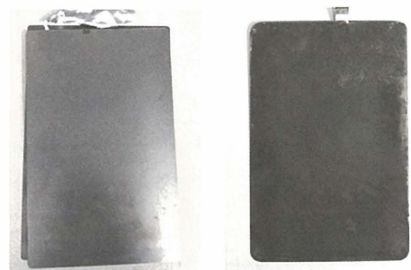
(a) Anode (b) Cathode (Black rust: Fe_3O_4 )
