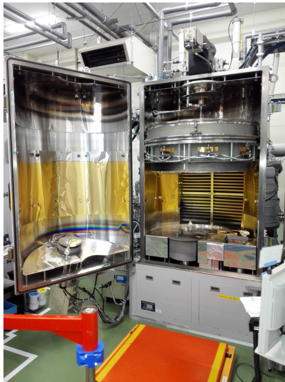
Figure 28: Evaporation machine of Etsumi company. Release of this photo has been permitted by the employee in charge of the deposition work.
