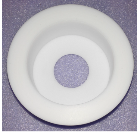
Figure 30: Crystal holder for the evaporation process.
