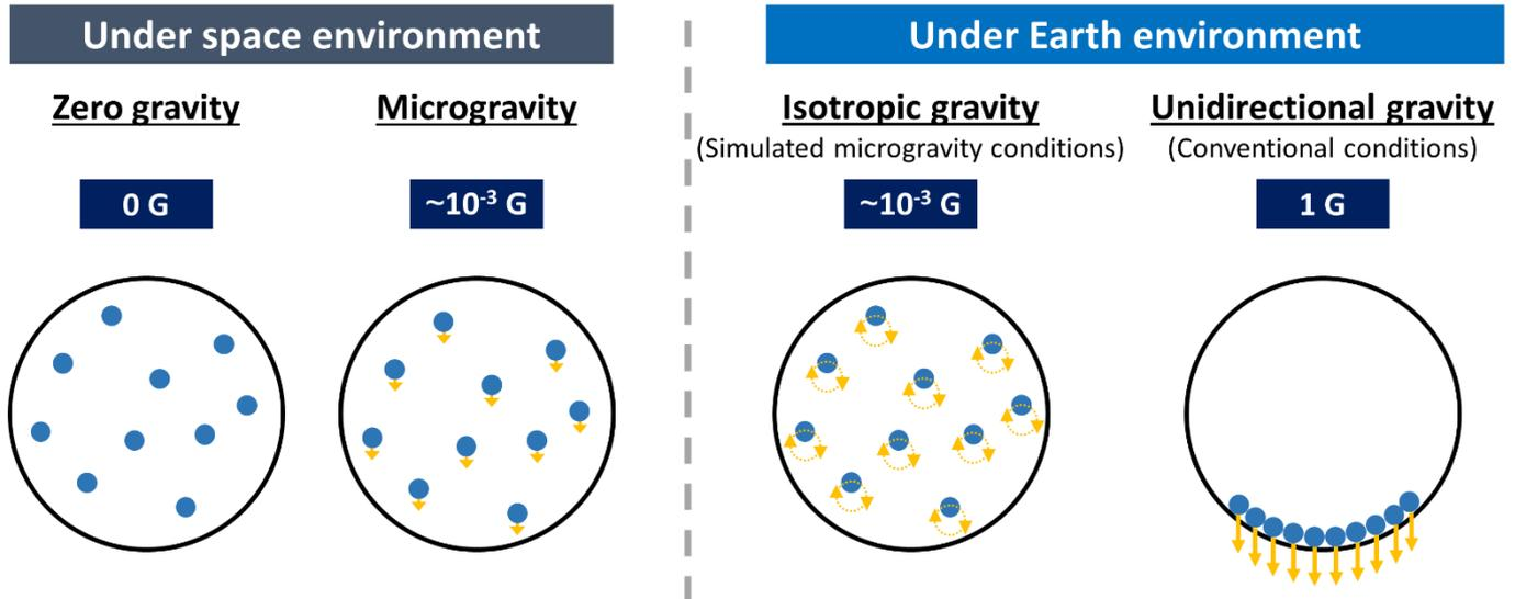
**Fig. 2** Comparison the effects of different gravitational environment on the physical phenomena of particle motion induced by the gravity, whereas particles have higher density than surroundings.
