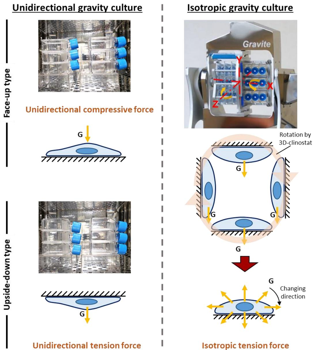
**Fig. 3** Culture systems using in this study, which are unidirectional gravity culture (left) with face-up type and upside-down type, and isotropic gravity culture (right) by operation of a 3D-clinostat (Gravite®) that generate the isotropic gravity culture conditions by rotations in X- and Z-axis with constant angular velocity.
