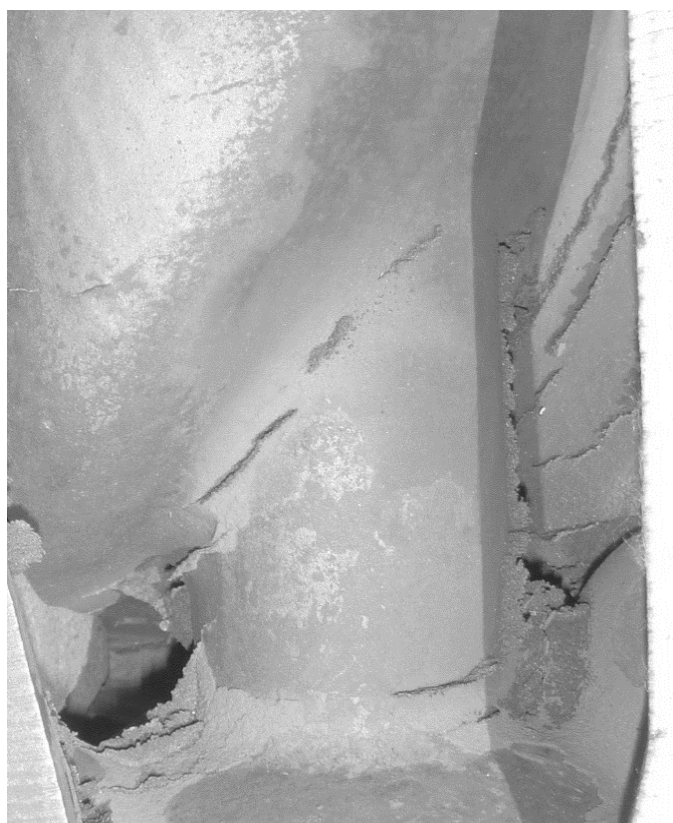
Fig.2-7. Veining defects on the surface of ductile iron that cast with furan self-hardening mold. (JIS FCD450-10)
