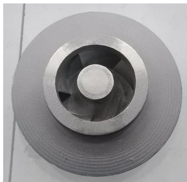
Fig.19 Cast impeller specimen with hollow structured core.
