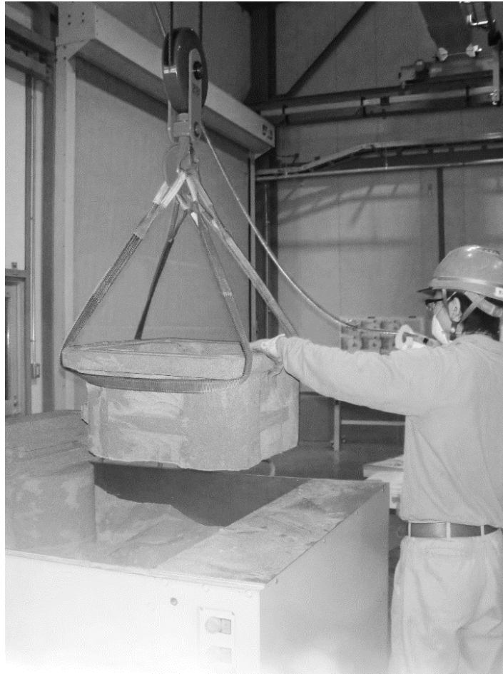
Fig.1-1 Photo of picking up an additive-manufactured sand mold (S-MAX, Exone). 1.26m 3 workspace is printed in 28h.
