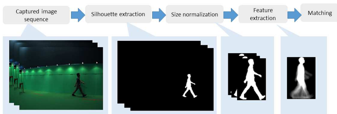
Figure 1.4: A general flow diagram for silhouette-based gait recognition.
