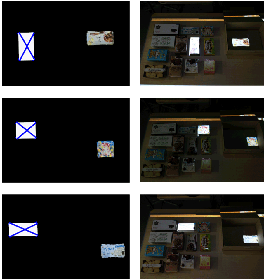
Figure 6.7: An Initial design of the packing instruction shows position of item to pick up, and final position and orientation of the item to be packed in a container.
