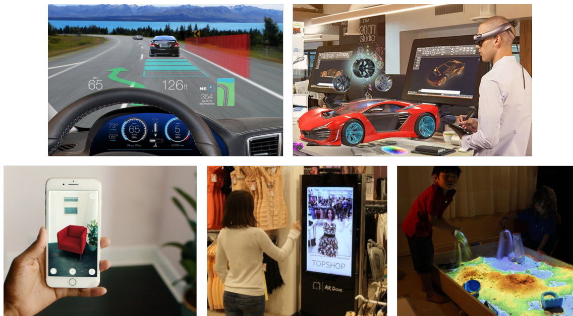
Figure 1.1: AR displays: head-up display, head-mounted display, handheld display, stationary display, and projected display (images taken from [10–14]).
