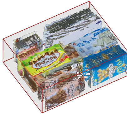
Figure 6.4: Simulated visualizations of a packing solution showing segmented point cloud data fit into the container.
