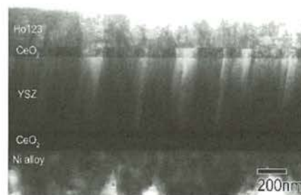
図6 \text{CeO}_2/\text{YSZ}/\text{CeO}_2 中間層の断面 Fig 6. Cross section of \text{CeO}_2/\text{YSZ}/\text{CeO}_2 buffer
