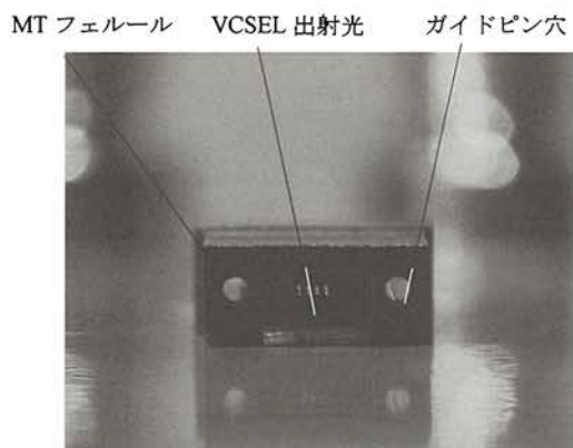
図11 表面実装用レセプタクルコネクタの正面写真 Fig.11 Photograph of the front face of the surface-mount receptacle connector.
