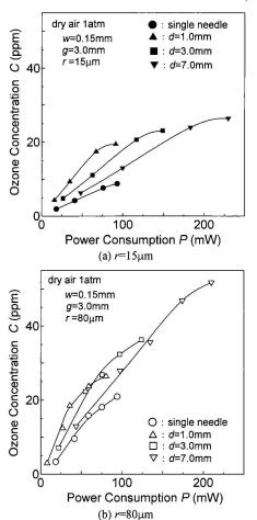
Fig. 5 Power consumption dependence of ozone concentration
