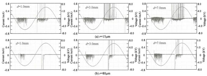
Fig. 8 Discharge current for various conditions (g=3.0mm, V=6.0kV)
