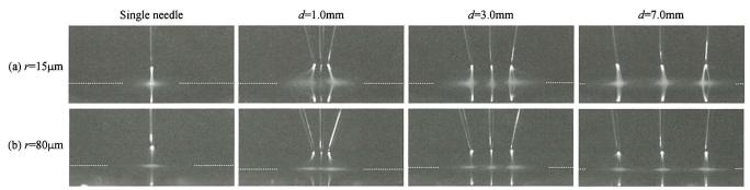
Fig. 7 Discharge imaged for multi-needles barrier discharge (g=3.0mm, V=6.0kV)
