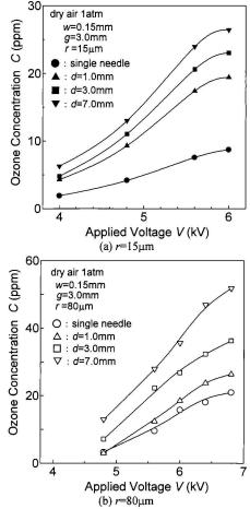
Fig. 3 Applied voltage dependence of ozone concentration
