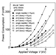
Fig.4 Relationship between applied voltage and power consumption
