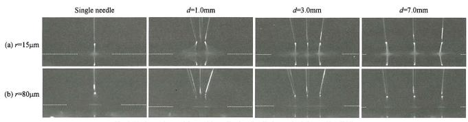
Fig. 6 Discharge imaged for multi-needles barrier discharge (g=3.0mm, V=4.8kV)
