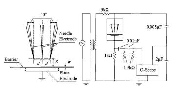
Fig.1 Electrode configuration
