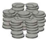
図3 ヘキサゴナルカラムナー相 Fig. 3 Schematic illustrations of hexagonal columnar (Col h ) mesophase.
