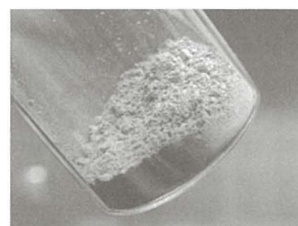
Fig.1 Reduced PANI synthesized by chemical oxidation
