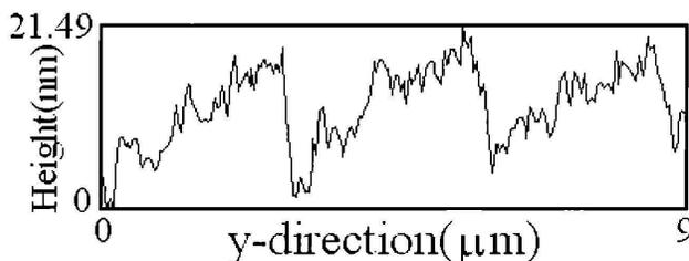
Fig. 6 Cross-sectional profile of the obtained resist grating.
