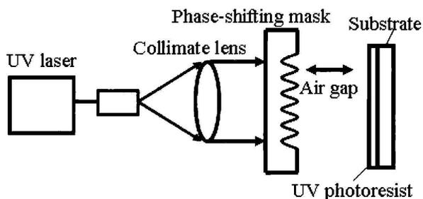
Fig. 5 Exposure layout with phase-shifting mask.
