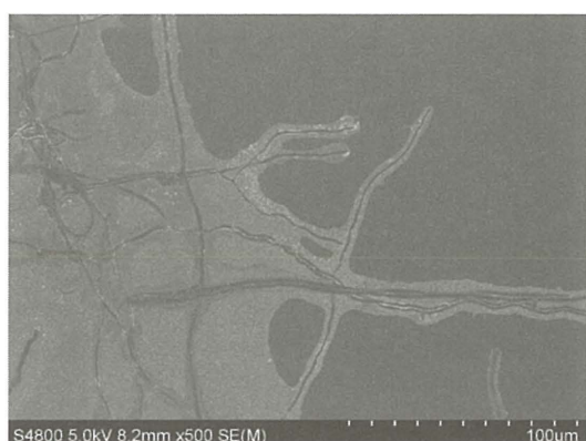
Fig.6(a) SEM image of the surface of the silica plate invaded by fungi, Fusariumoxysporum .
