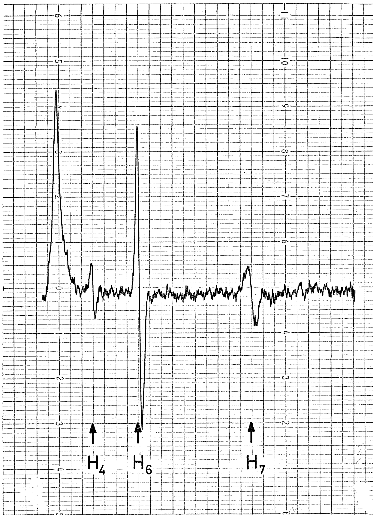
Fig. 6 Typical result of cross relaxation measurement. H_4 , H_6 and H_7 represent harmonic fields (see notation in Fig. 1).
