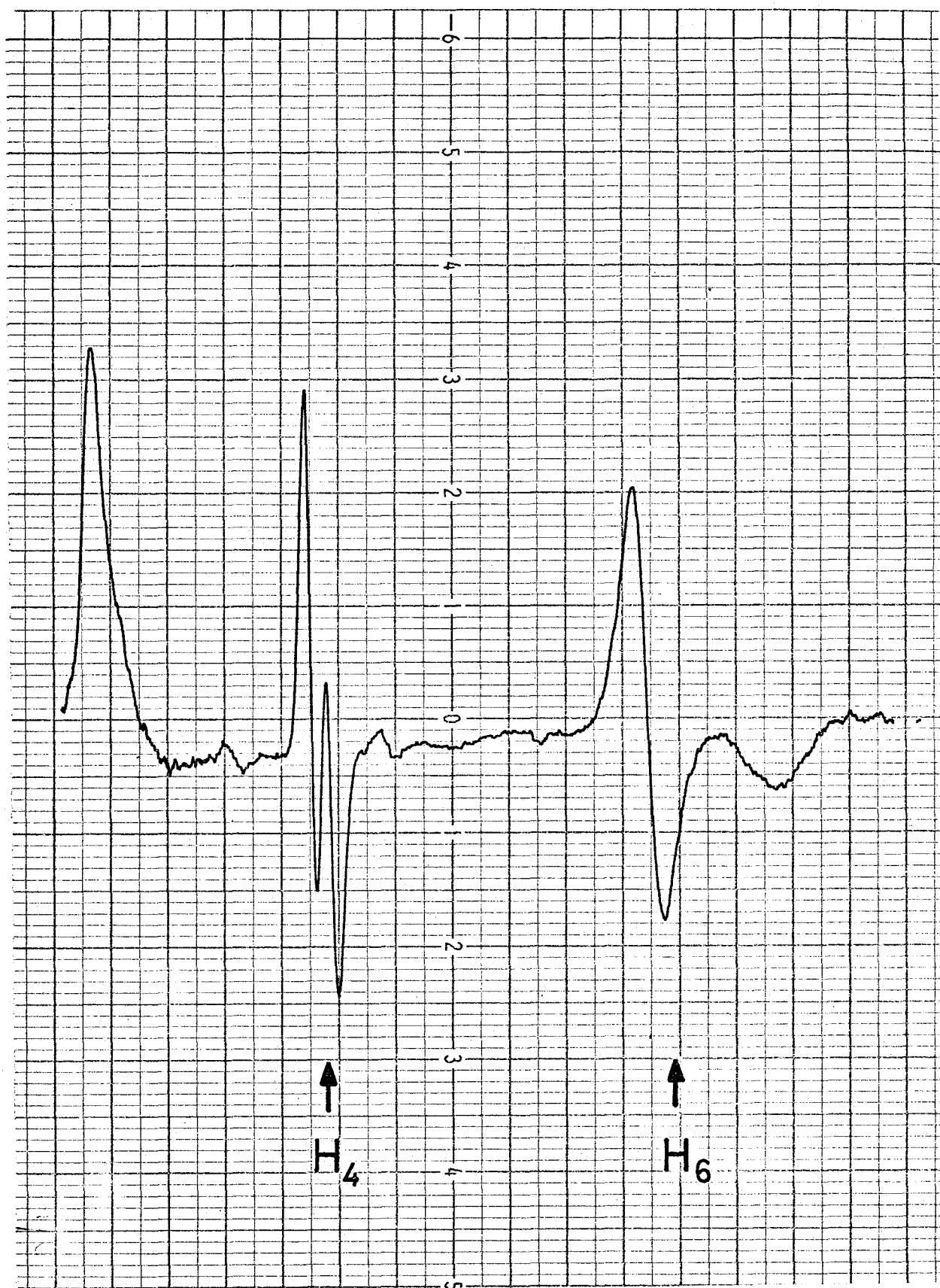
Fig. 8b) Cross relaxation signals for false single-crystal. ( \theta \sim 70^\circ )
