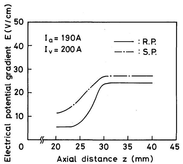
Fig. 4 Axial distance dependences of electrical potential gradient at different arc polarities.
