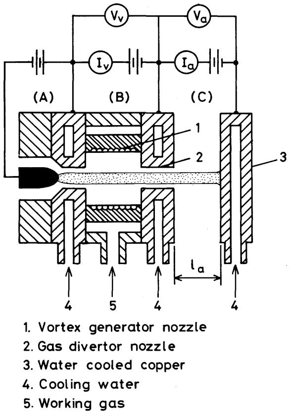
Fig. 1 Schematic diagram of the plasma arc generator.
