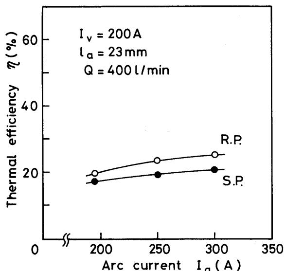
Fig. 8 Effects of arc current on thermal efficiency.
