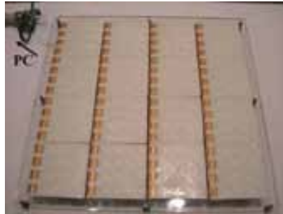
Fig. 4 A large-area tactile sensor system fabricated by integrating the stretchable sensor sheets and the self-organized network of distributed processors (256 channels).
