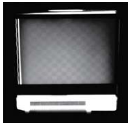
Figure 2 Ultralow power liquid crystal displays operated at 3 V with NAOS-SiO 2 /CVD-SiO 2 stacked gate oxide.
