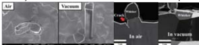
Fig. 5 The growth mechanism of Tin whiskers by inflicting thermal cycling in air and vacuum.
