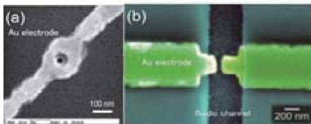
Fig.2 SEM images of (a) a surround gate and (b) an in-plane nanopore device with control electrodes. There is a nanopore at the center of the surround gate.
