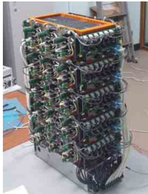
Fig.1. Solid-state switch for the klystron modulator of the L-band electron linac using SI thyristors.
