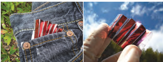
Fig. 2 Foldable solar cell based on nanopaper.
