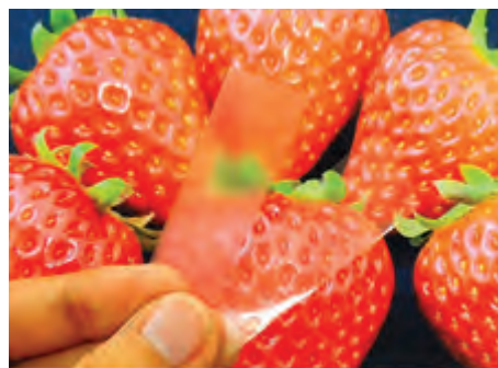
Fig. 6 Translucent and transparent nanopaper from high-concentration dispersion.
