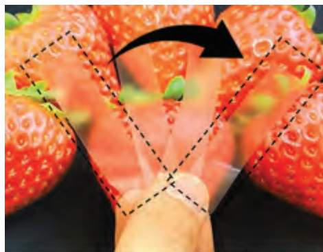
Fig. 4 Transparent nanopaper by high-humidity heating.
