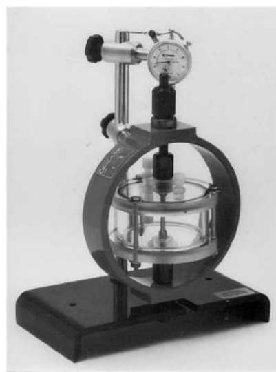
Fig. 1-4: NACE TM0177 method A (Tensile test). [8]
