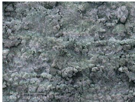
Fig. 3-9: Surface morphologies of corrosion products on material 95A after corrosion test for 720 h.
