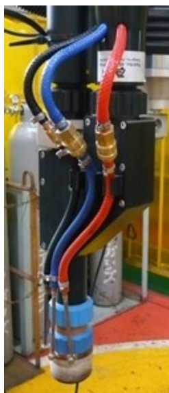
Fig. 2.1 Duplex current feeding MIG torch.
