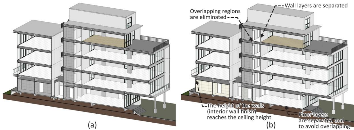
Figure 4.21 Three-dimensional section views of (a) the original BIM model and (b) the manually modified BIM model for case study 2.
