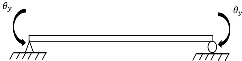
Fig 2. 5 Simply supported beam model for static analysis
