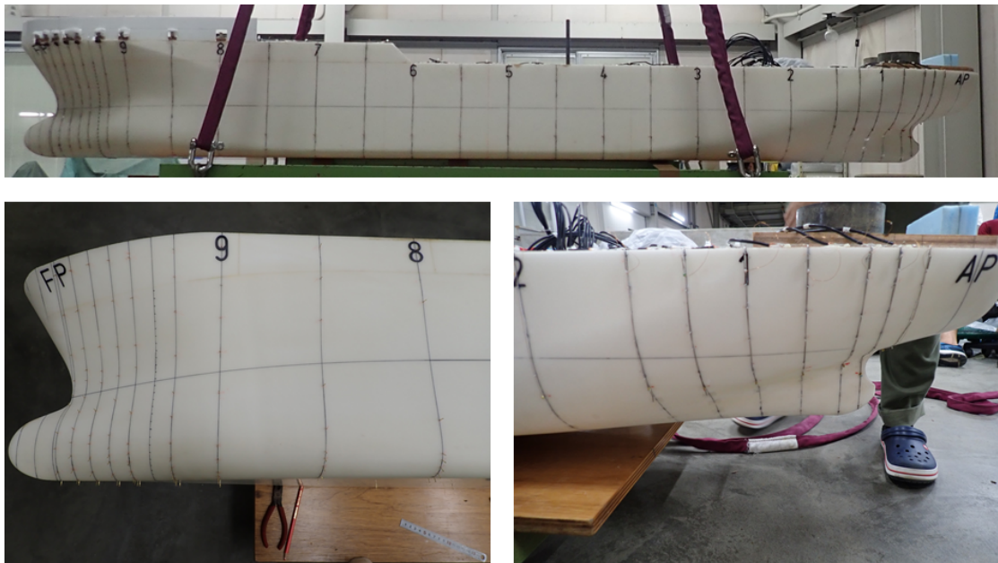
FIGURE 2.1: RIOS bulk carrier model for ship-side wave measurement
