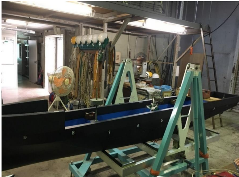
Figure 3: Adjustment of the Radius of Gyration
