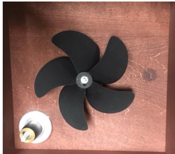
Figure 2: Propeller model for 3.2 m KCS model ship
