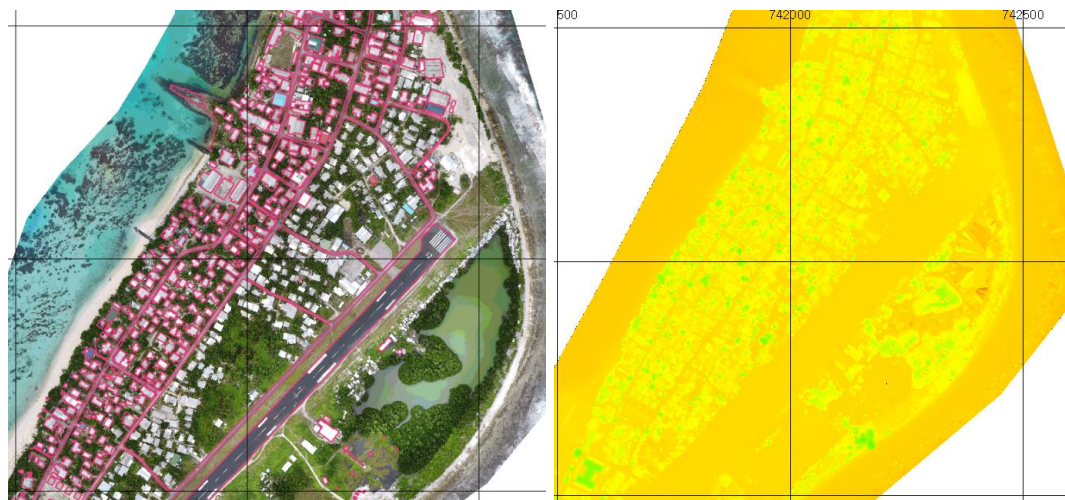
Figure 2.8: Combining UAV survey result and field survey data (left: visual inspection result, right: DSM result)
