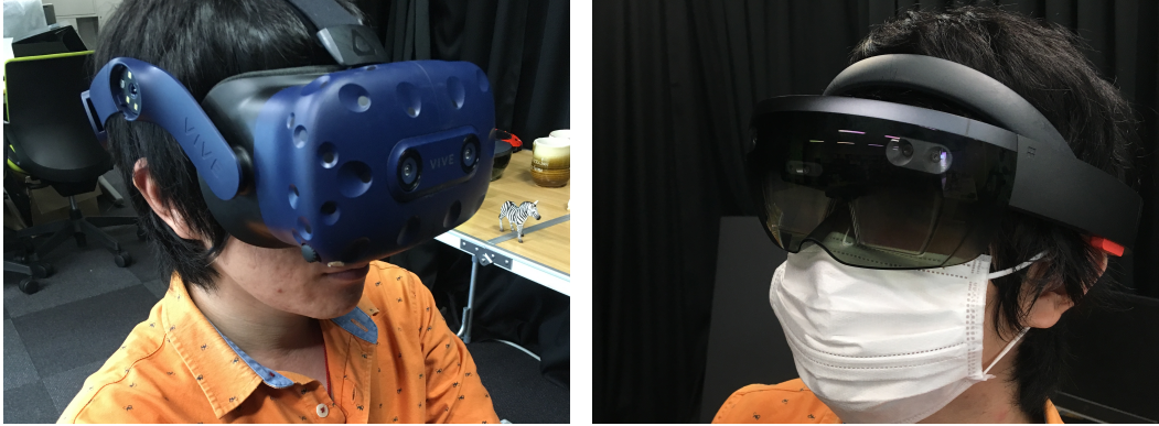
Figure 1.1: Sample images of immersive HMDs and OST-HMDs. Left: A user wearing an immersive HMD which provides the user with a fully-immersive VR experience and hence prevents the user from directly viewing the real world. Right: A user wearing an OST-HMD which renders digital content directly in the user’s field of view overlying the real world.
