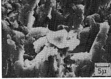
Photo. 2 Scanning electron micrograph of included particle in emery paper (1000 grade).
