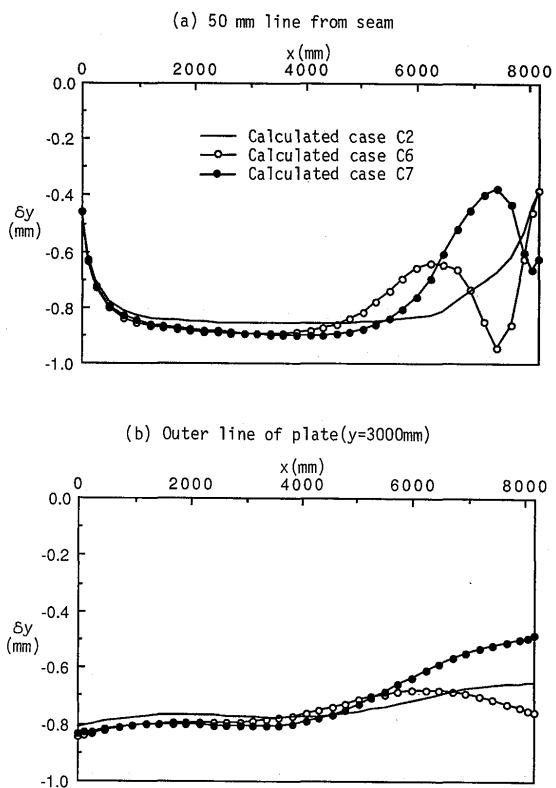
Fig.13 Influence of local heating on the shrinkage
