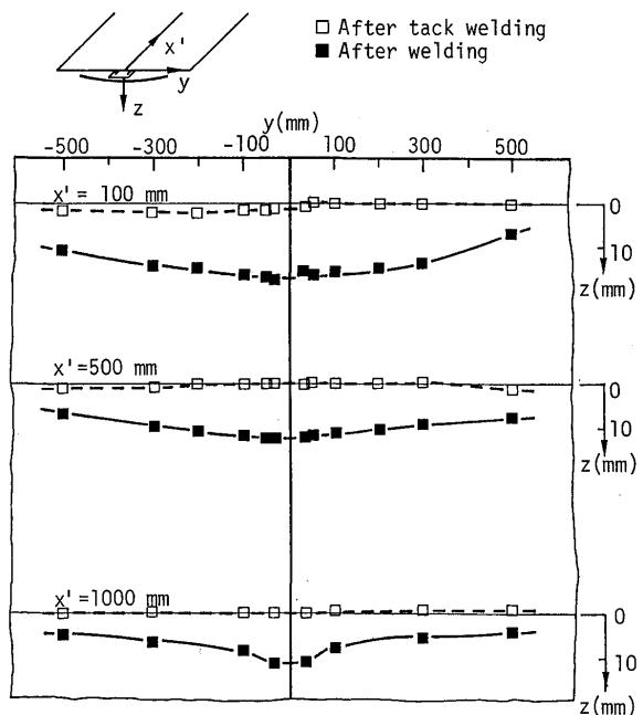
Fig.3 Measured deformation of welded plate
