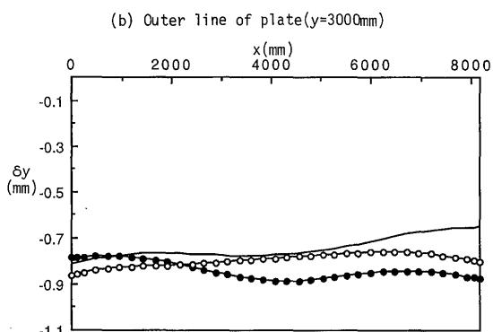
Fig.15 Influence of welding sequence on the shrinkage
