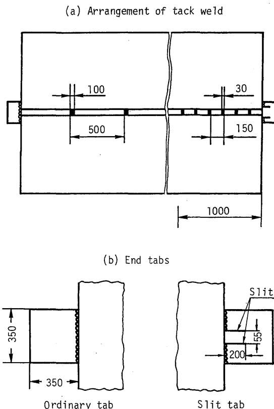
Fig.1 FCB Welding method (case E1~E4)
