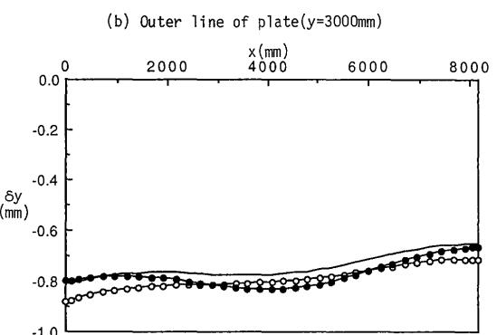
Fig.17 Influence of roof gap on the shrinkage
