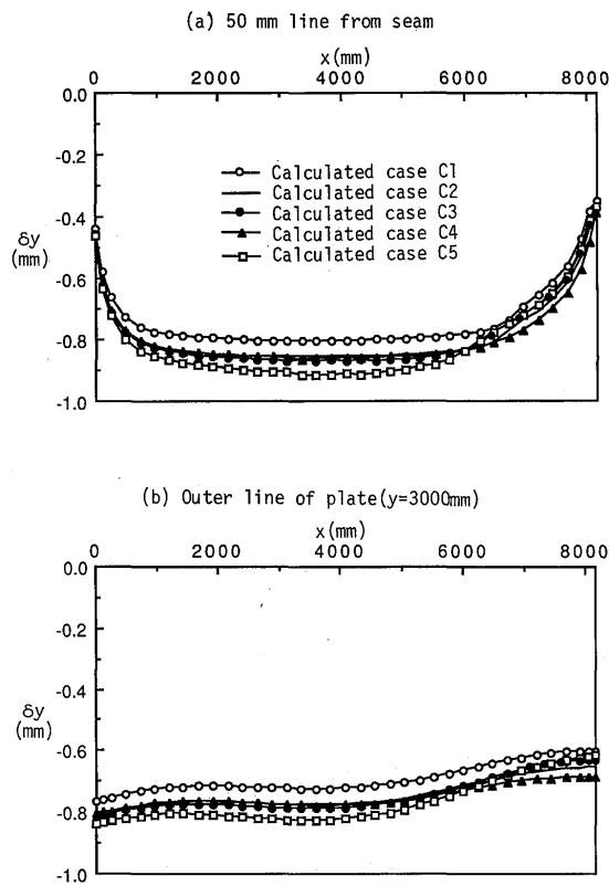
Fig.10 Influence of restraints of groove on the shrinkage
