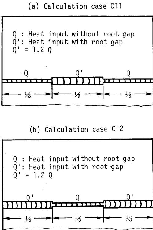
Fig.8 Idealization for analysis of root gap effects
