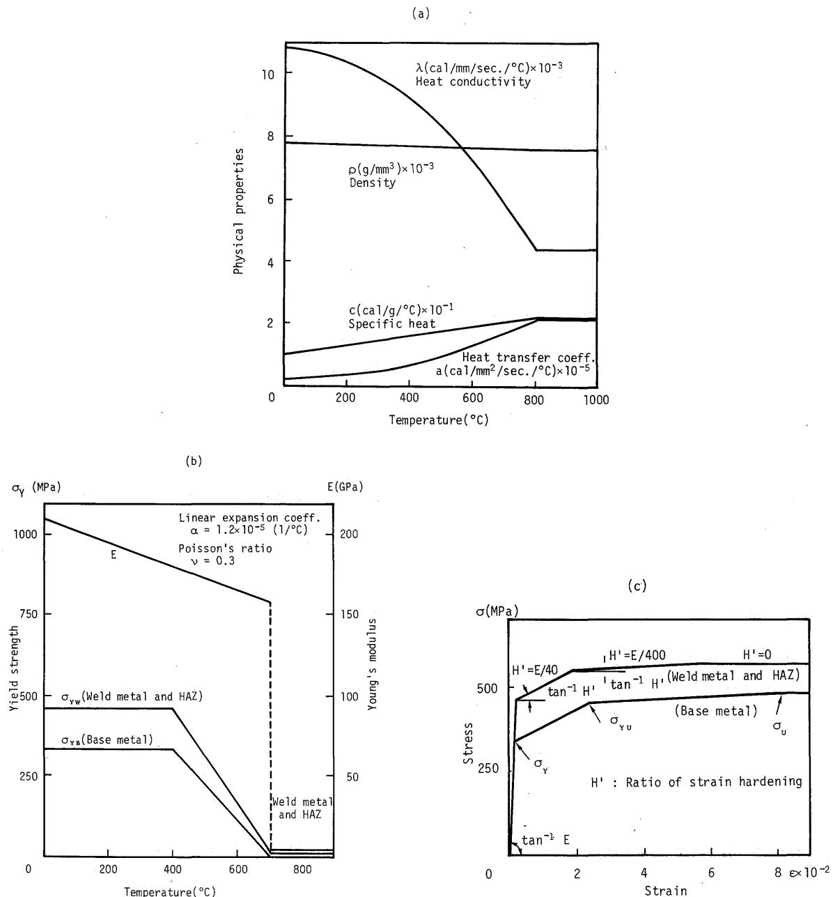
Fig.6 Temperature dependency of physical and mechanical properties
