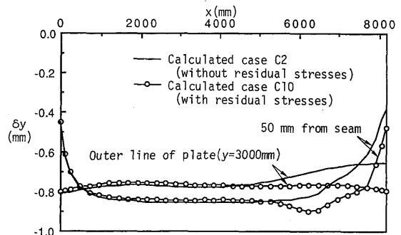
Fig.16 Influence of residual stresses on the shrinkage
