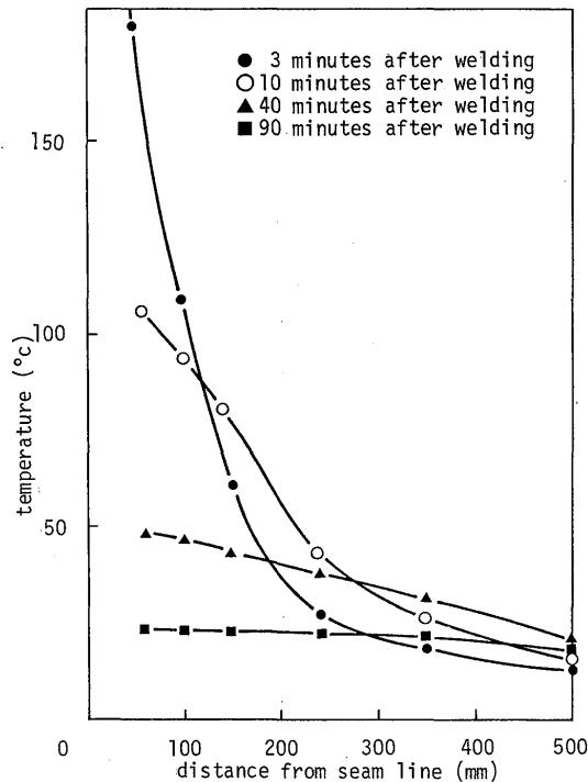
Fig. 4 Temperature distribution after welding
