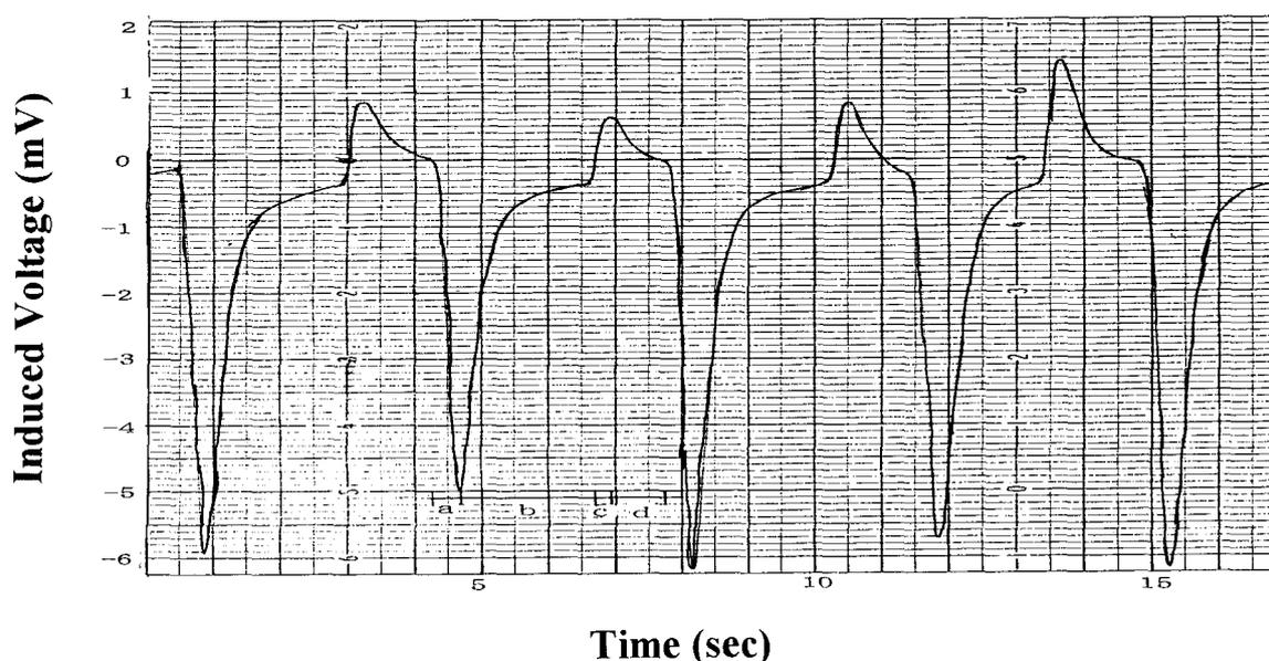
Fig.6 Response curves on the induced voltage by pulling at the fullerene doped PUE films.
