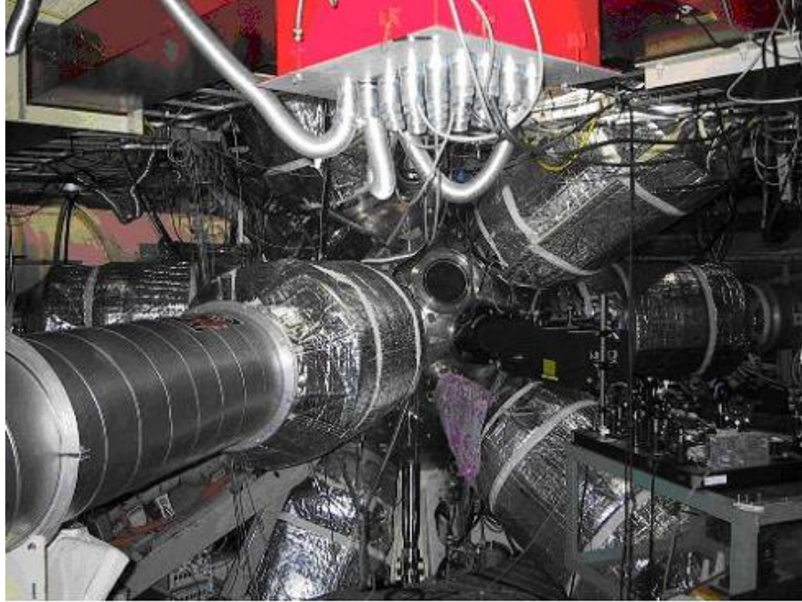
Figure 2-2: Chamber I. Beams are induced into the chamber from different directions to adapt multiple experiments.
