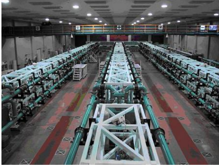
Figure 2-1: The Gekko XII system. There are 12 beams in Gekko XII facility, with 1053-527 nm in Chamber I. Pulse duration ranges 0.1 ns - 4 ns. Usually 3 or 4 shots are possible for 12 beams experiment.
