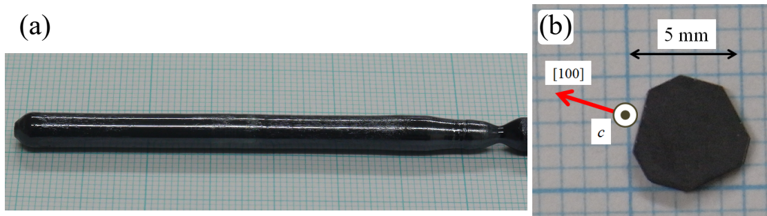
Figure 3-2-4: (a) Synthesized single crystal rod of \text{BaCo}_2\text{V}_2\text{O}_8 obtained by the FZ method. (b) Plate-shaped single crystal sample of \text{BaCo}_2\text{V}_2\text{O}_8 viewed from the c -axis.
