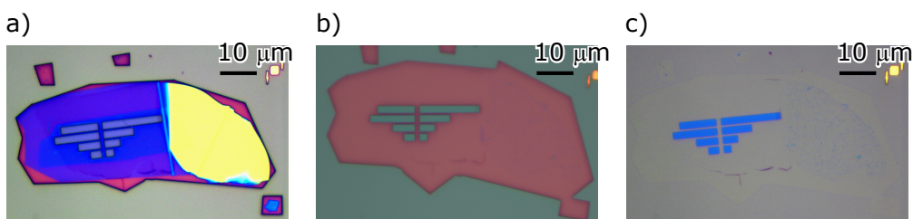
FIGURE 6.7: Hall bar etching process of hBN/graphene/hBN stack.
